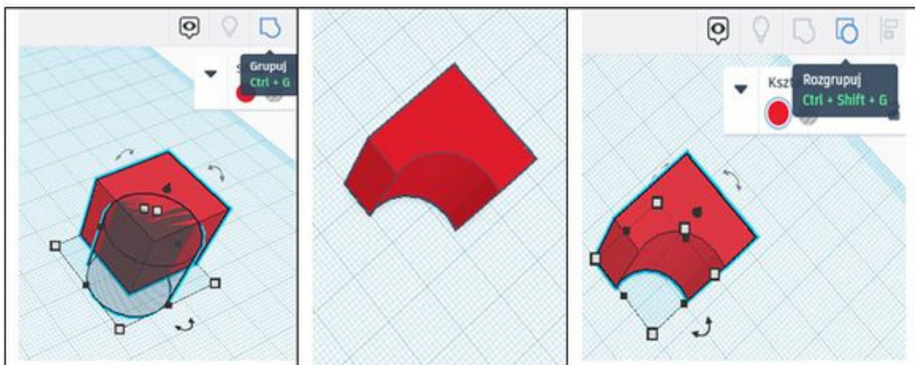
Figure 30. Subtraction (cutting out) of solids Source: own work using the Tinkercad program
